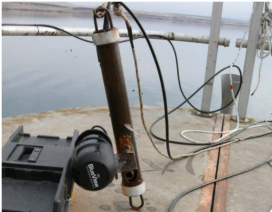
Figure 2.3. BlueView Sonar Attached to Trolley and Ready for Deployment
